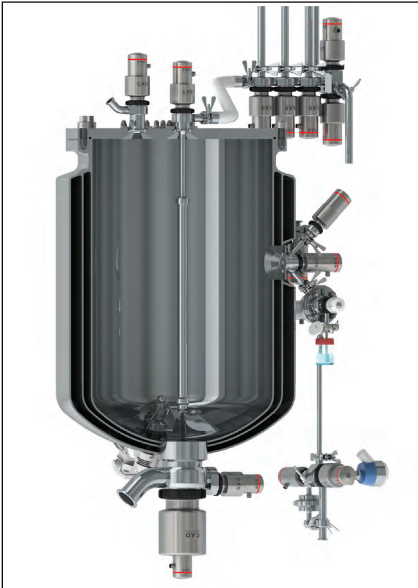
Figure 8 – Bringing it all together: The multi-function device and well thought out valve cluster allows for multiple feed stream into the vessel utilizing the same port. By feeding various process streams in with such a device, splashing is eliminated. Reducing the required ports significantly improves the cleaning and sterilizing of the vessel. Rendering courtesy of Rattiinox Srl.
