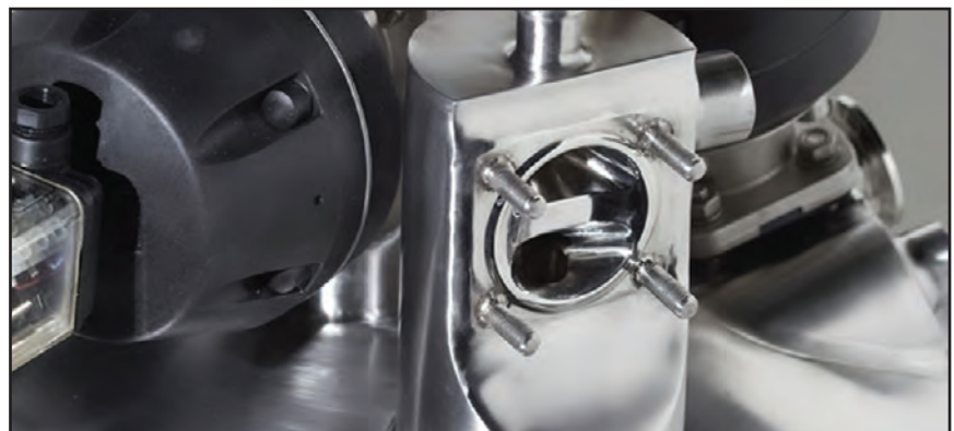
Figure 5 – Vessel air vent fabrication. The design adds a significant and nearly impossible to clean dead leg to the vessel top. In addition, the internal welds would be impossible to polish, contributing a significant risk to proper cleaning. Image courtesy of the internet.
