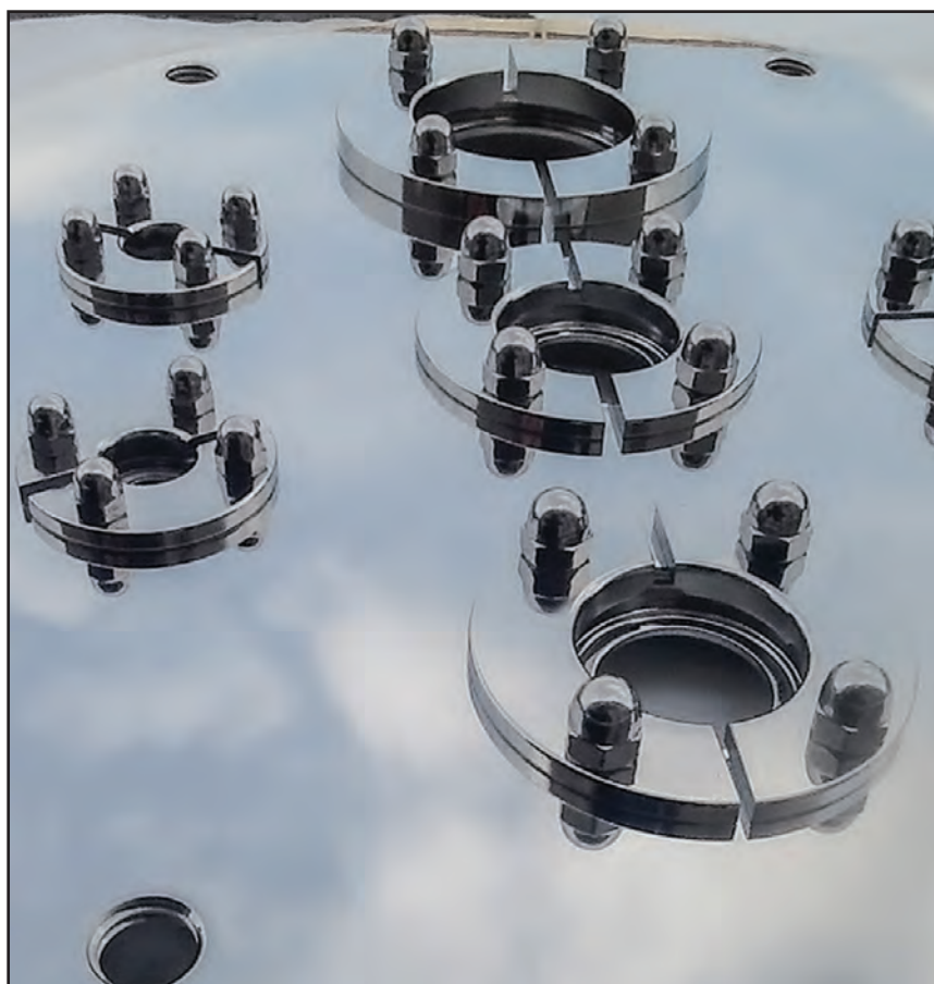
Figure 3 – Aseptic process vessel with zero dead leg couplings machined into the vessel top plate. No welding allows for flexibility with positioning of port locations. Image courtesy of the author.
