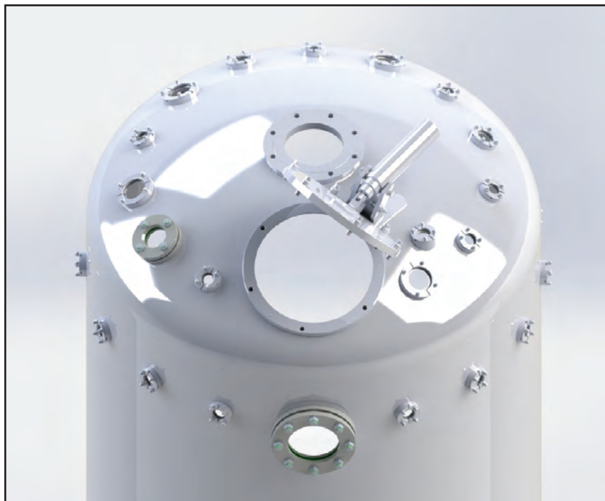
Figure 1 – Low profile zero dead leg flanges positioned both radially and vertically on vessel top eliminate potential shadow areas and significantly reduce the risk associated with insufficient cleaning with a spray device. Rendering courtesy of EMA Engineering.
