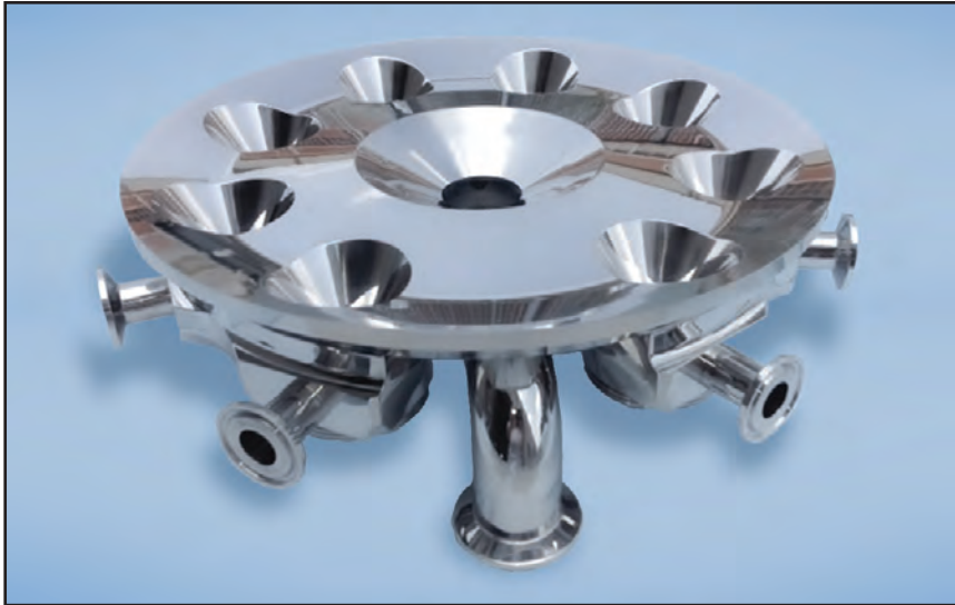
Figure 4 – Aseptic filling vessel with multiple outlet valves machined from solid. The feed valves to the filler and the special drain contours are machined into the bottom dish which will be welded to the vessel. The configuration ensures even flow to the filler and complete draining. Image courtesy of the author.
