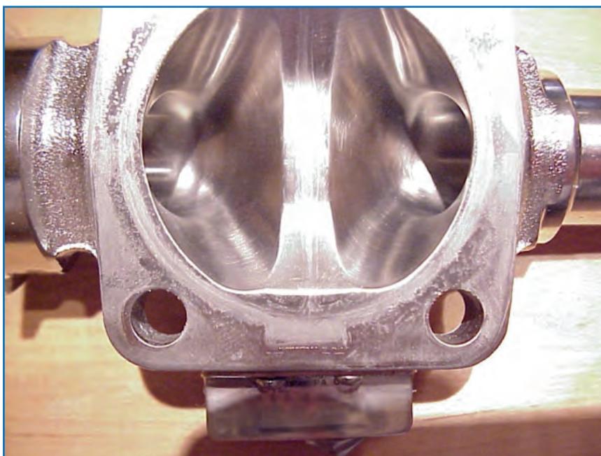
Figure 5. The area between the body edge and where the diaphragm seats. This is a common area for entrapment of product even after cleaning. This image is from a valve that was never installed. The EPDM diaphragm left residue behind that clearly shows it was seating behind the body edge.
