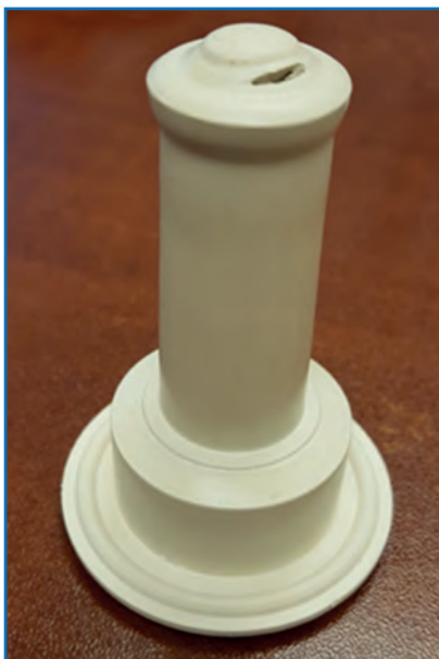
Figure 3. TA failed silicone diaphragm from a first generation radial valve – failure attributed to diffusion bubble rupture.
