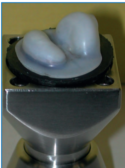
Figure 4. Deformation of fluoropolymer diaphragm face due to vacuum conditions while hot. The image also shows deformation of EPDM backer due to compression set.
