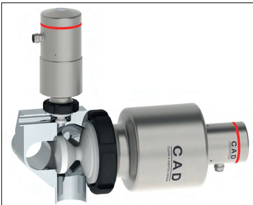
Figure 6: Whether single-use based valve or stainless steel valve, distributing high purity water or water for injection (WFI) to vessels remains a common step. Maintaining loop and distribution leg integrity is vital. The advantage of a modular approach is evident in this design shown here. The main take-off valve and the optional downstream steam/nitrogen valves are machined as part of the main pipe up to 4". The assembly is very compact and free of dead legs. Pneumatic actuators and position indicators are optional.
